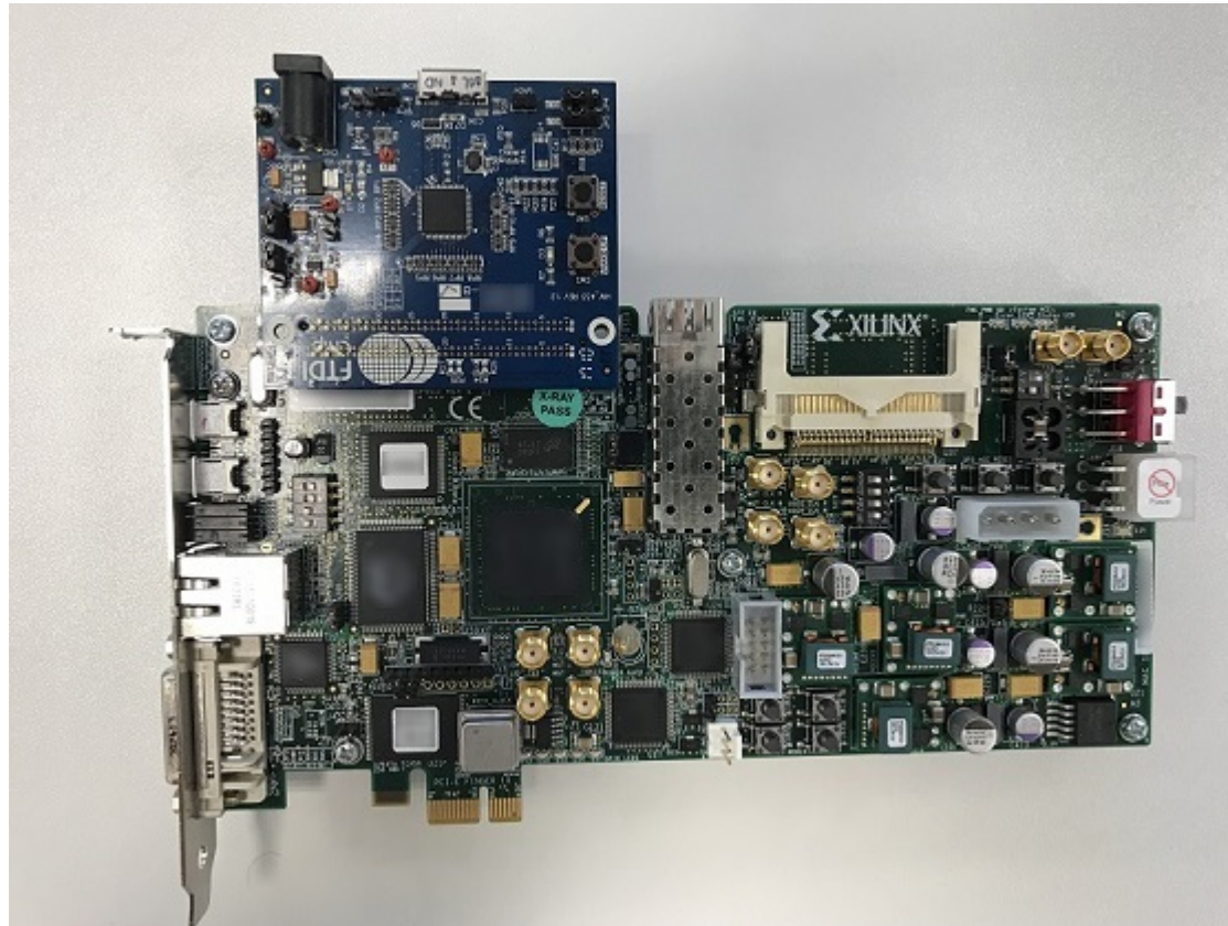
FPGA Spartan-6 FPGA SP605[10] + FTDI ft601[11] USB 3.0
