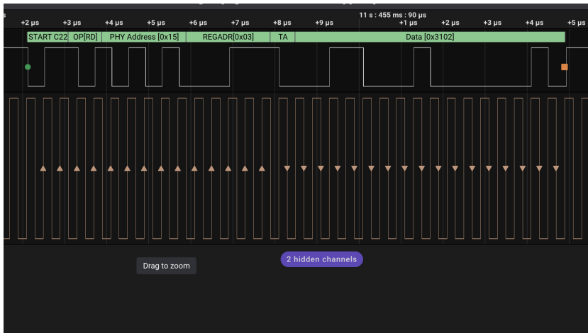
Fig. 8. MDIO bus signals
